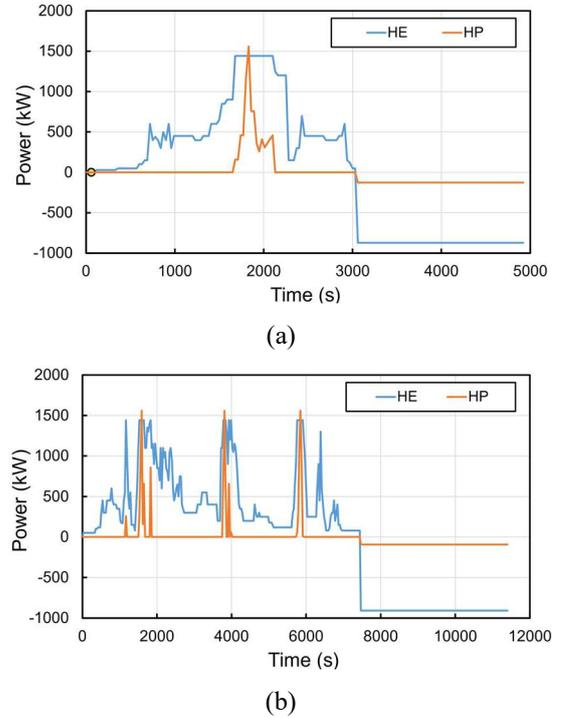
Fig. 11. Optimal power sharing between HE and HP battery pack for parallel full-active topology, (a) Primary profile, (b) Secondary profile
