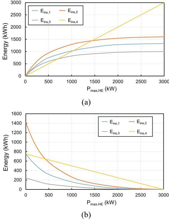
Fig. 8. Energy to be installed to meet the design criteria, (a) HE battery (b) HP battery.
