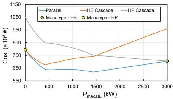
Fig. 9. Cost of monotype and HESS topologies at different values of  $P_{max,HE}$ .
