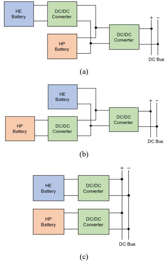
Fig. 4. HESS topologies considered in this work, (a) HE cascade full-active, (b) HP cascade full-active, (c) parallel full-active.
