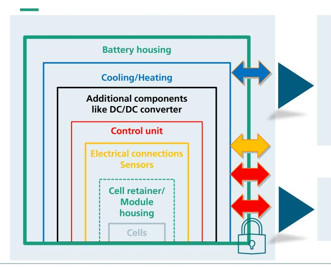
The **battery space** shall be **adequately ventilated** (to prevent accumulation of flammable gas) **and cooled** in such a way as to maintain the specific set of environmental design conditions.
