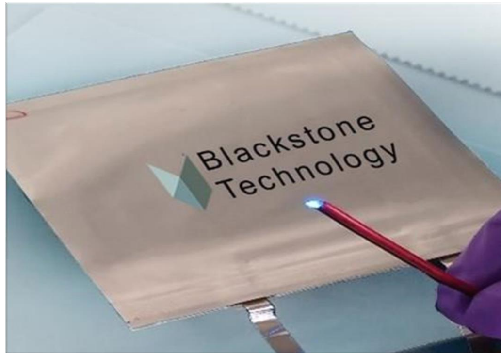
Working lab demonstrator of a 3D printed all solid state battery
